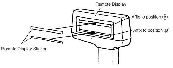
Affix the remote display stickers to the inner edge of the remote display sheet. (The sticker should be affixed on both the operator side and customer side)
